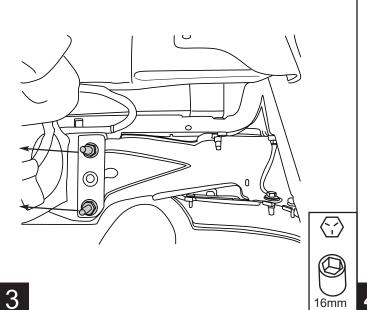
Torque to 41 ft-lbs / 55Nm 9 **Note:** Use provided sleeve nut (13) with washers (14) when short studs are present.
