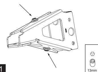
В Torque to: A) 33 ft-lbs / 44 Nm B) 16 ft-lbs / 22 Nm 15mm
